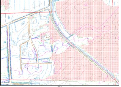
of data for photogrammetrically derived points (on left) and LiDAR mass points (on right). Because of the point density, breaklines are not as critical to accurately model the terrain. Arguably, breaklines are still required to identify man-made changes to drainage patterns such as bridges and culverts for hydrologically-enforced elevation models.
